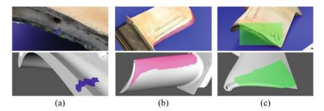
Fig. 7.6 3D defects: a crack (polyline) b spallation (polygon) c material loss (bounding box)
