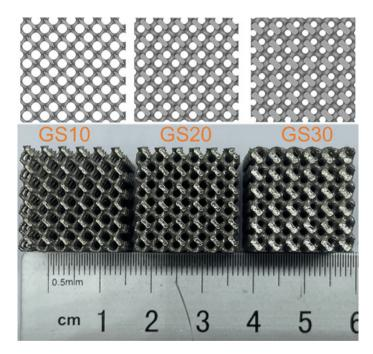
Fig. 9.2 Ti6Al4V GS manufactured by L-PBF
