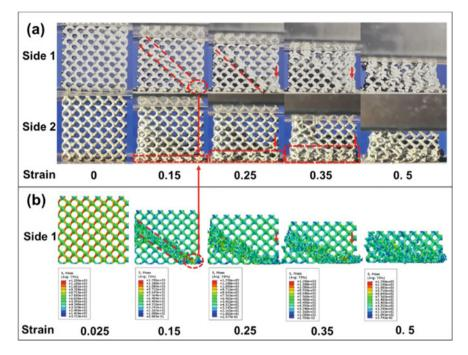
Fig. 9.5 Experimental and simulated failure modes of GS10
