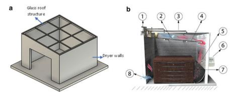
**Fig. 1.4** Drying oven configuration. **a** Drying oven structure. **b** Drying oven parts: (1) fan, (2) temperature sensor, (3) glass roof, (4) solar absorption metal plate, (5) humidity sensor, (6) automatic control box, (7) wood to be dried, (8) air exhaust vents
