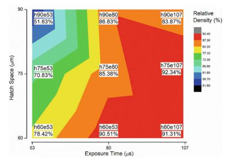
Fig. 13.3 Effect of hatch spacing and exposure time on relative density
