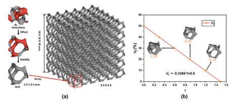
Fig. 9.1 a Modeling process of GS and b relationship between the volume fraction  $V_f$  and offset parameter t for GS
