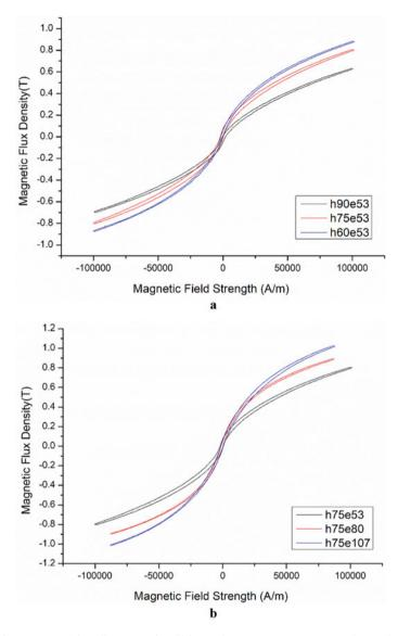
**Fig. 13.4** B (T)–H (A/m) diagrams of FeSi6 samples: **a** constant exposure time (53  $\mu$ s) with different hatch spacings, **b** different exposure time with constant hatch spacing (75  $\mu$ m)
