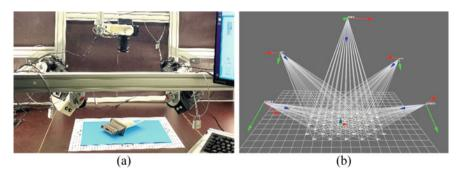
Fig. 7.4 a Optical feature inspection system (OFIS) b virtual OFIS calibration
