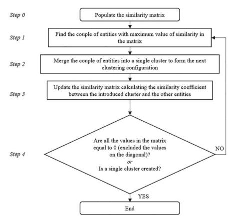
Fig. 22.1 Flowchart of the hierarchical clustering algorithm
