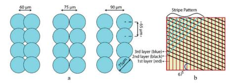
Fig. 13.1 Scanning strategies: a hatch spacing values, b scan pattern and angle between layers
