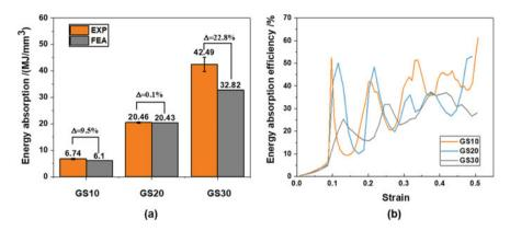
Fig. 9.6 a Energy absorption and b energy absorption efficiency of GS
