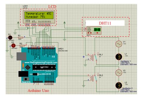
Fig. 1.3 Electronic system of the drying oven
