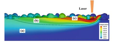
Fig. 18.3 Three zones existed in LPBF process a heat-affected zone, b transition zone, and c the melt pool
