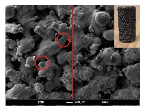
Fig. 13.6 SEM images of top and side view of h75e80 sample and photo of the h75e80 sample
