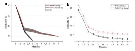
Fig. 1.5 Comparison between the natural drying process and solar oven drying. **a** HC versus time observations. **b** ANOVA graph
