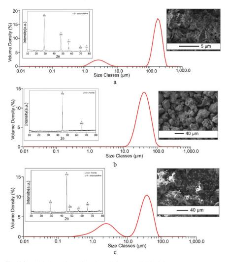
Fig. 13.2 Particle size analyzes of powders a Si, b Fe, c FeSi<sub>6</sub> blended
