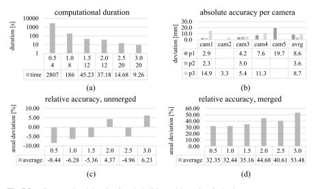
Fig. 7.8 a Computational duration for admissible mesh/step sizes b absolute accuracy per camera c relative accuracy, unmerged 3D annotations d relative accuracy, merged 3D defects
