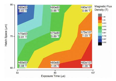
Fig. 13.5 Effect of hatch spacing and exposure time on magnetic flux density
