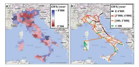
Fig. 21.2 Mapping of critical energy areas and energy flows on the electrical grid for 2040. **a** Energy deficit and surplus by province. **b** Energy flows on high-voltage grid connections
