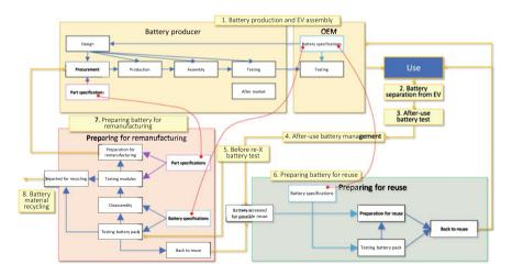
Fig. 6.1 A simplified view of the circular life cycle of batteries and battery material with a focus on reuse and remanufacturing
