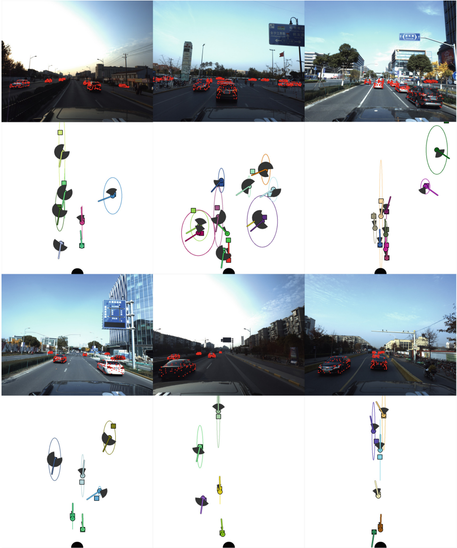
Fig. 5. Visualizations of estimated pose and uncertainty. Circles show the estimated positions of cars, squares are ground truth positions of these cars, colour rays show ground truth yaw angles, grey fans show the estimated one-sigma yaw range. Ellipses visualise one sigma position uncertainty (Color figure online)
