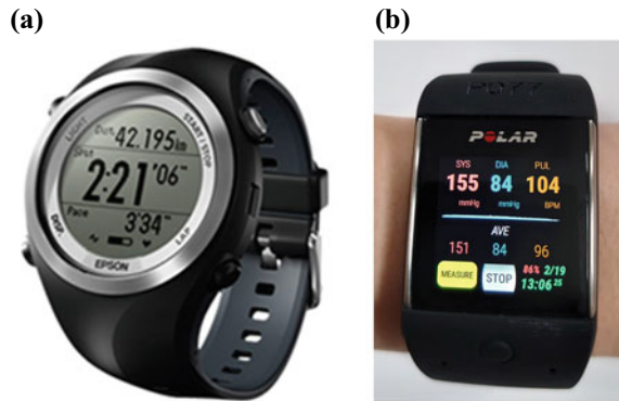
Fig. 2 Wearable device for a pulse rate measurement ( http://www.epson.jp/products/wgps/sf710s/ ) and b DCBP estimation
