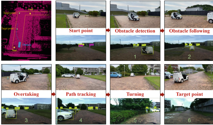
Fig. 6. On-site testing scenarios and distribution of the stages.
