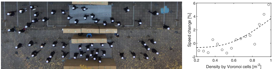
Fig. 4 Left: Configuration used to test the steering efficacy on the bidirectional flow over “long” time periods. Right: Change in average speed against the baseline condition (without optical sheet) for different densities. Only the straight sections are considered in this analysis. Each dot is computed for a density bin of 0.05 \text{ m}^{-2} .
