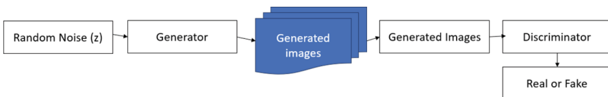
Fig. 1. Flow diagram of proposed Convolutional based GAN
