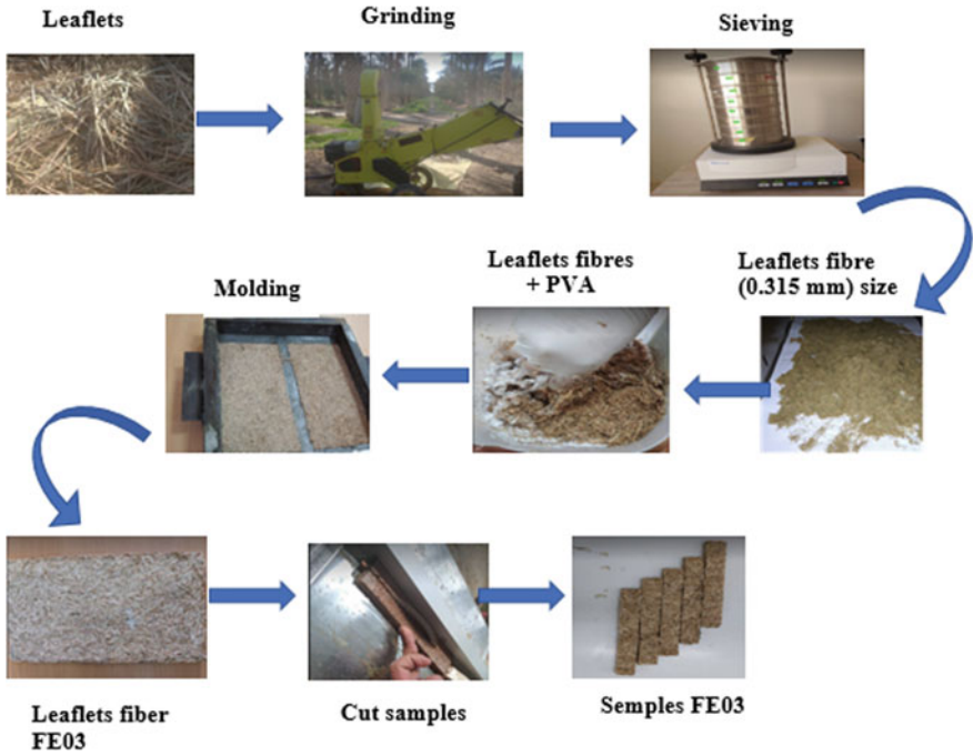
Fig. 1 Experimental procedure to obtain the bio-composite material samples
