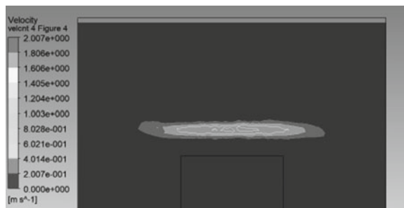
Fig. 13 Velocity contour on YZ plane at 15 h
