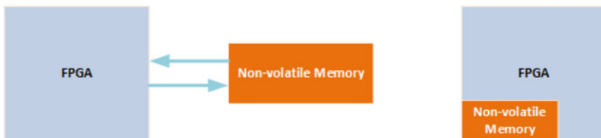
Fig. 11.10 Illustration of FPGA master mode configuration (left for external memory, right for internal memory)
