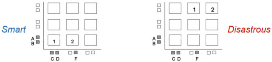
Fig. 10.11 FPGA placement matters
