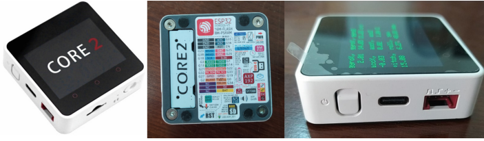
Fig. 3. M5Stack Core2 ESP32 IoT Development Kit.
