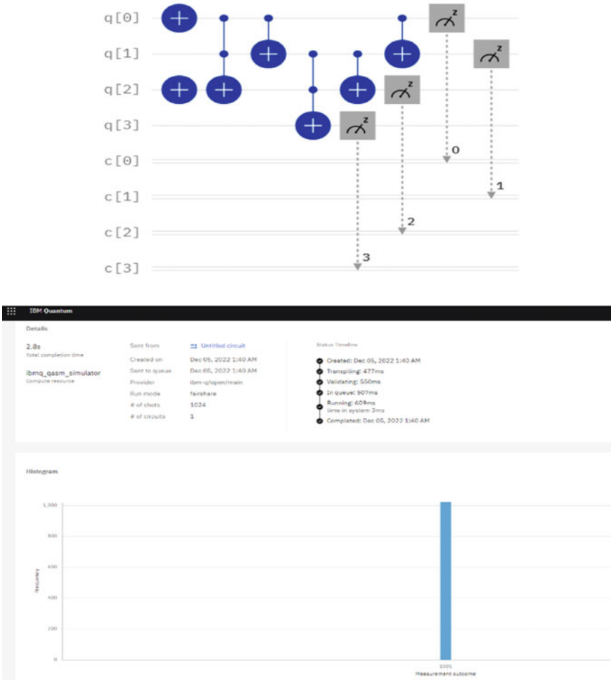
Fig. 10 Full adder implementation using simulation Qiskit simulator
