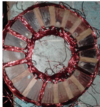
(b) Pancake-shaped air-core stator with distributed winding .
