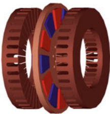
(a) Dual-stator and single-rotor topology of Axial-flux permanent magnet generator.
