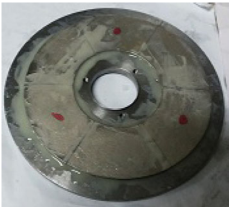
(a) Permanent magnet pasted on the rotor.
