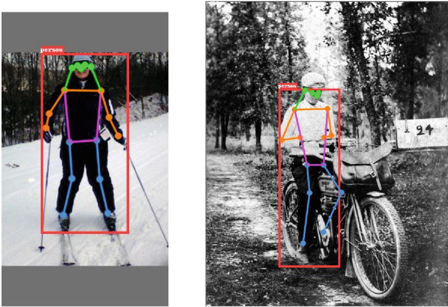
Fig. 1. Example of keypoint inference of images in the COCO dataset by YOLO.
