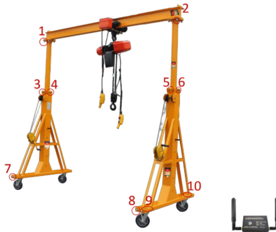
Fig. 2. Damage identification of gantry crane.
