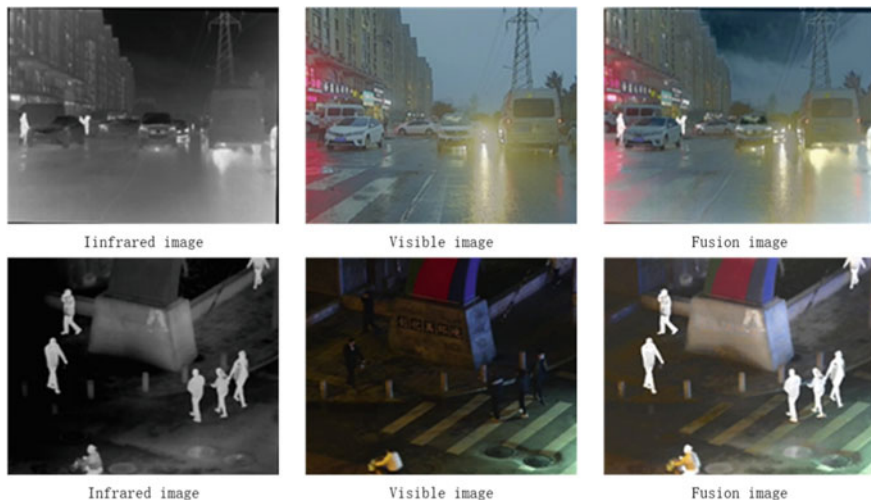
Fig. 2 1 Left: IR image 2 middle: RGB image 3 right: fusion image
