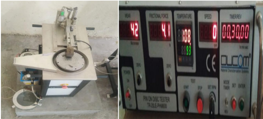
Fig. 2 Experimental setup of pin-on-disc for measurement of wear and force (frictional)
