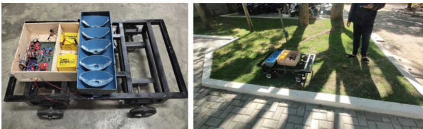
Fig. 7 Components assembly and operation test of small robot for water spinach planting
