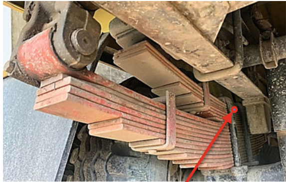
The position of the broken leaf spring
