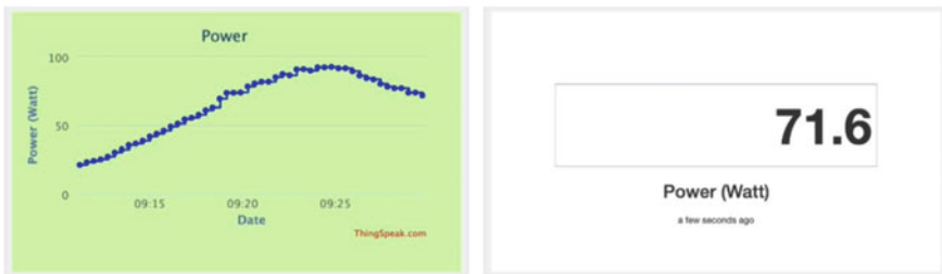
Fig. 5 Power output battery measurement of solar panel system
