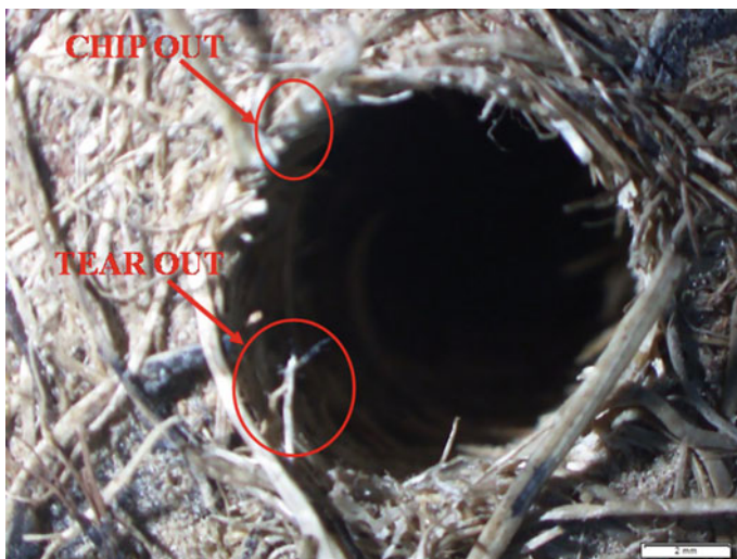
Fig. 5 Hole image captured at the top of particleboard surface
