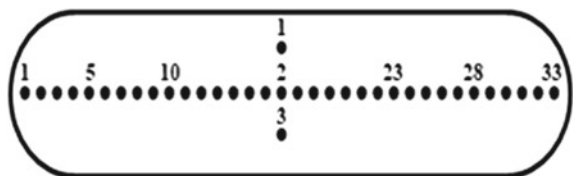
Fig. 8 Hardness test point on leaf spring
