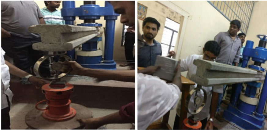
Fig. 4 Moment on a precast column
