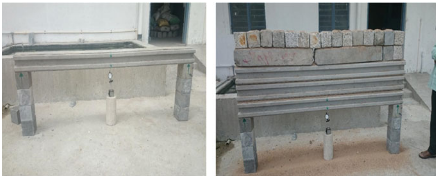
Fig. 2 Flexural testing of precast beam elements
