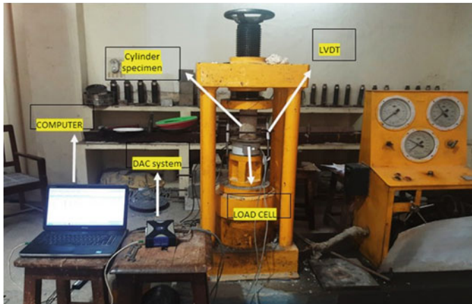
Fig. 1 Testing of cylinder specimen under compression for stress–strain behavior
