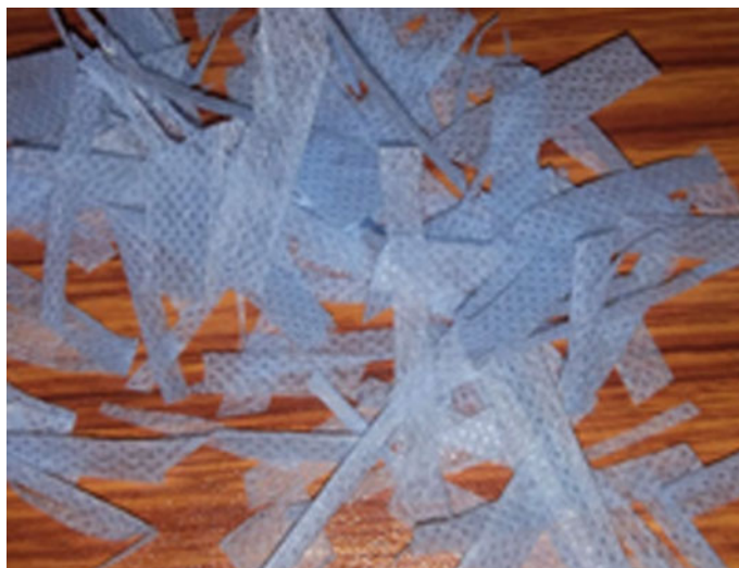
Fig. 1 Single-use face mask shredded into 2 cm × 0.5 cm
