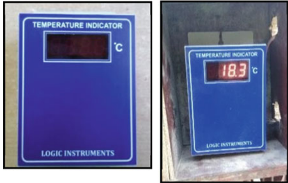
Fig. 13 Digital temperature monitor and concrete placing temperature
