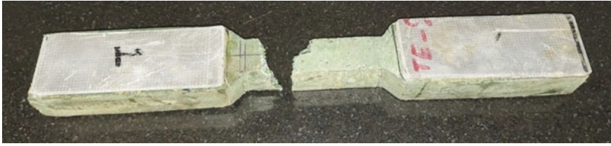
Fig. 7 Failure pattern of dog-bone shaped Specimen in tensile test
