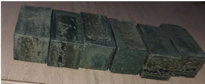
Fig. 14 Squared Prism shaped recycled plastic lumber specimens
