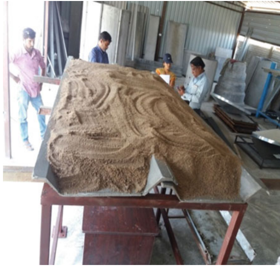
Fig. 1 Flexural testing of precast roofing sheets
