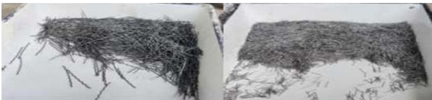
Fig. 1 Steel fibres 50 and 12.5 mm
