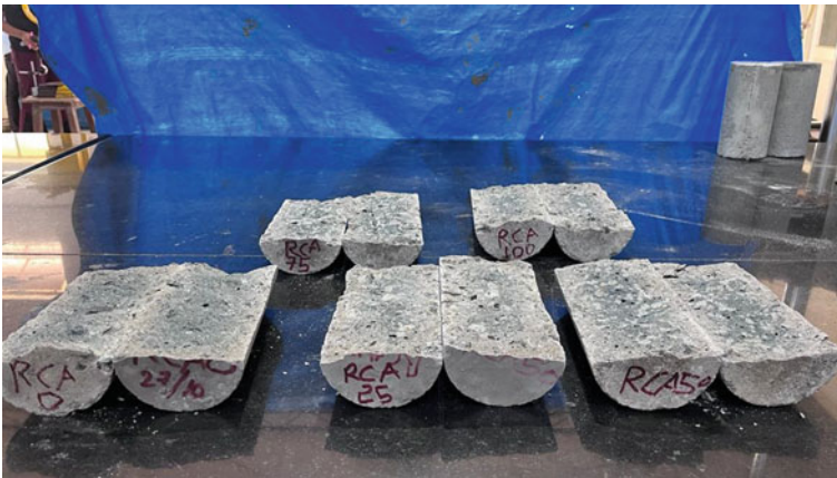
Fig. 8 Failed samples after splitting tensile strength test
