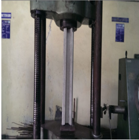
Fig. 3 Uniaxial compression of precast column elements
