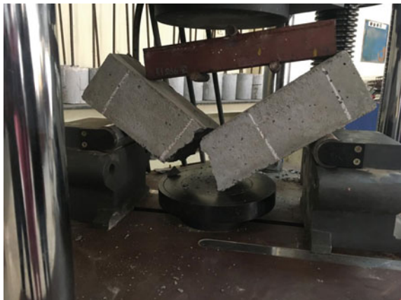
Fig. 8 Failed samples after splitting tensile strength test
