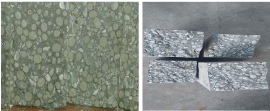
Fig. 11 Failure mode of FAAC
