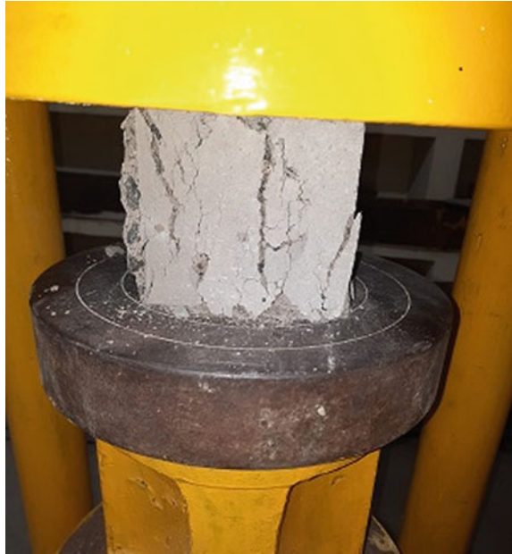
Fig. 7 Testing of specimens in compression
