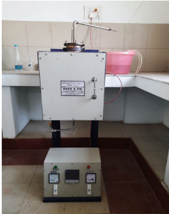
Fig. 1 Pyrolysis reactor for production of biochar
