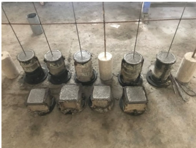
Fig. 2 Specimens cast in moulds
