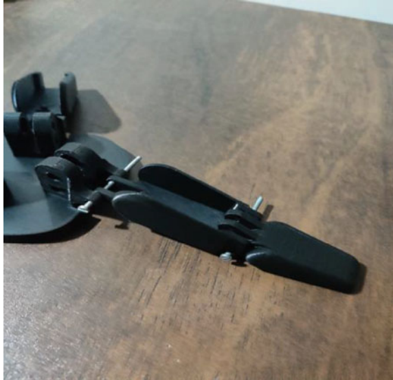
Fig. 10. 3D printed parts of modified gripper
