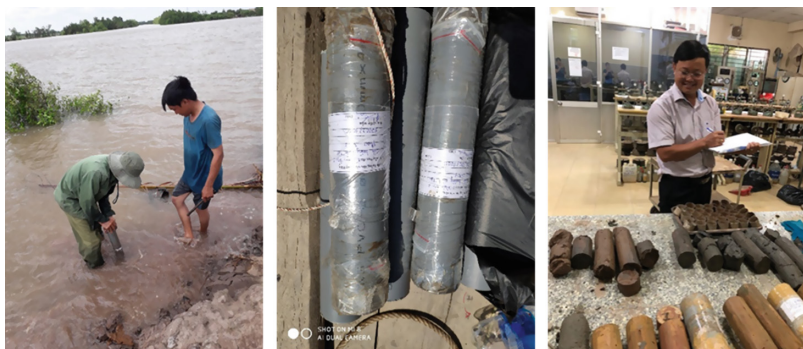
Fig. 3. Soil samples and laboratory analysis for bank material characteristic
