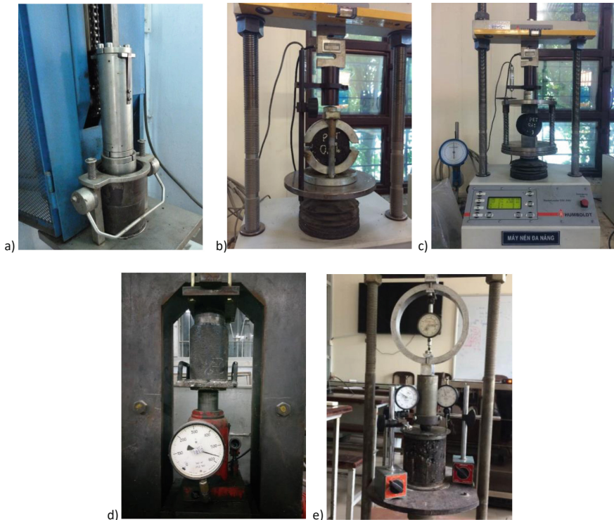
Fig. 3. Set-up for all tests in this study: a Marshall compactor; b Set-up for Marshall test; c Step-up for indirect tensile strength test; d Sample preparation for static resilient modulus test; e Set-up for static resilient modulus test.
