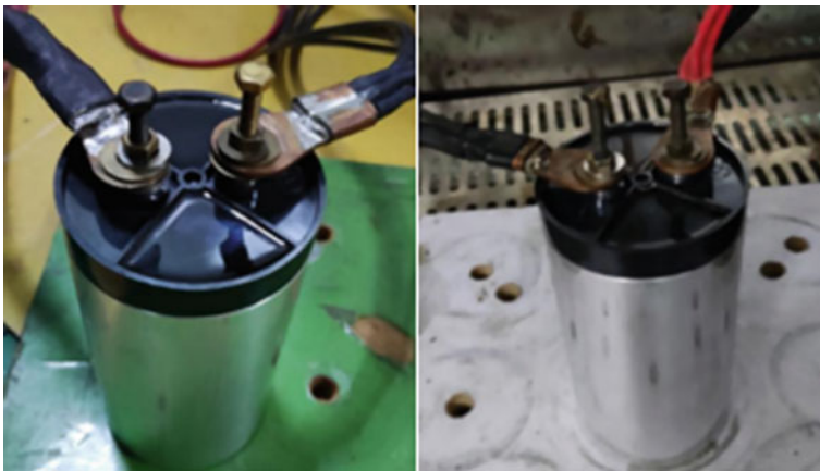
Fig. 4 7.5 \mu\text{m} capacitor withstand voltage test diagram
