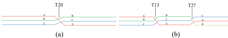
Fig. 2 Schematic diagram of conductor transposition a incomplete transposition, b complete transposition
