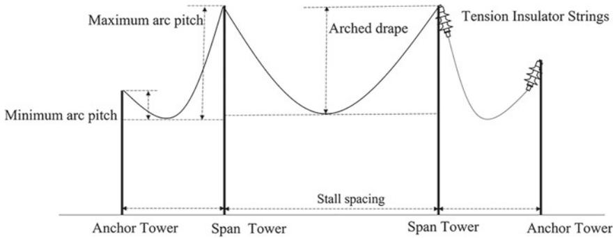
**Fig. 1** Section diagram at the crossing point
