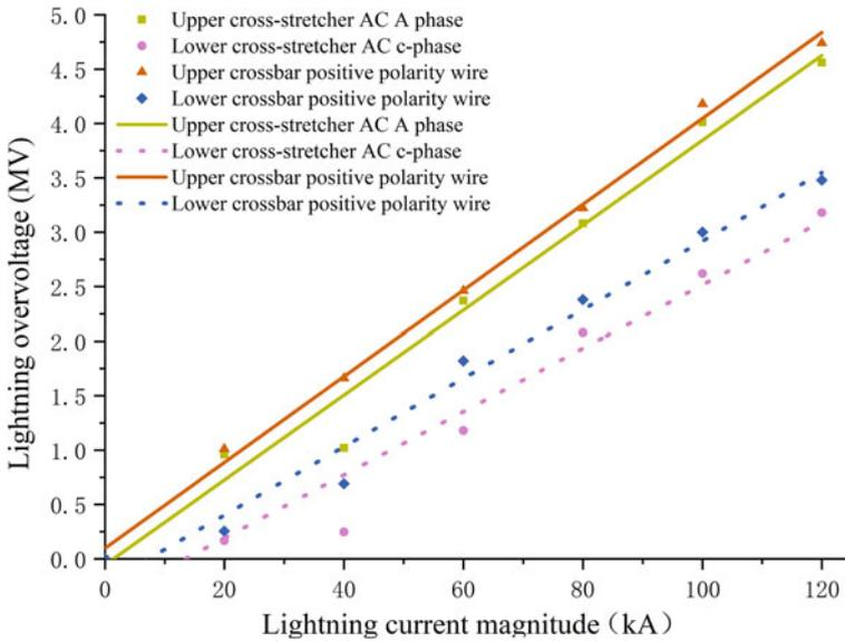
Fig. 6 Different lightning currents hit the upper transverse transmission line
