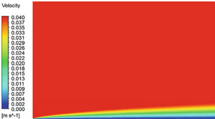
Fig. 7 Cloud chart of wall velocity distribution
