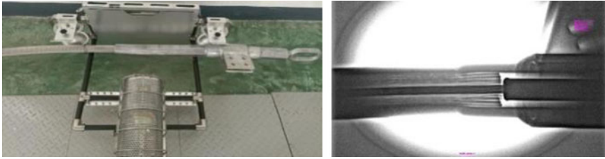
Fig. 7 Test layout and imaging diagram of NY-1250/100 tension clamp sample
