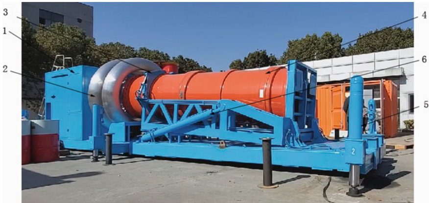
Fig. 1 AC voltage resistance test platform (horizontal). 1. Rain cover, 2. Voltage balancing ring of reactor, 3. Hoop, 4. Reactor, 5. Extended hydraulic support leg, 6. Hydraulic cylinder
