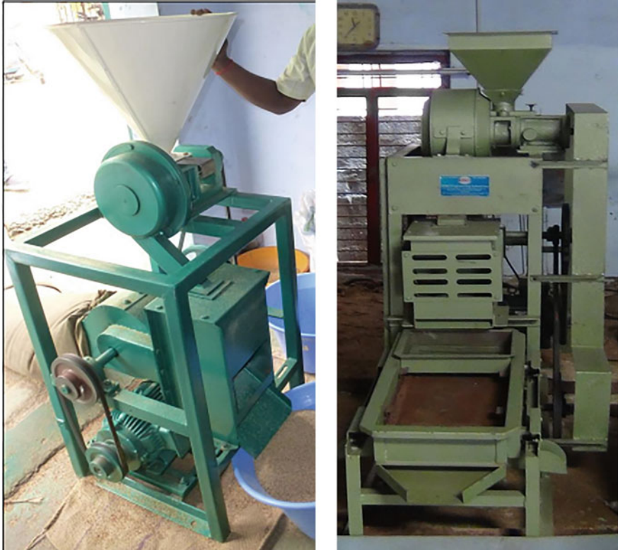
Fig. 6.2 Victor single-chambered CF dehuller (left) and AVM single-chamber CF dehuller with grader (right)
