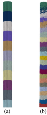
Fig. 5. Fuel stack status in Case P80C40-1: (a) before relocation, stack height = 480 mm, (b) after relocation, stack height = 408.59 mm. Only upper part of the fuel stack was shown, and the cladding was hidden for better visualization.
