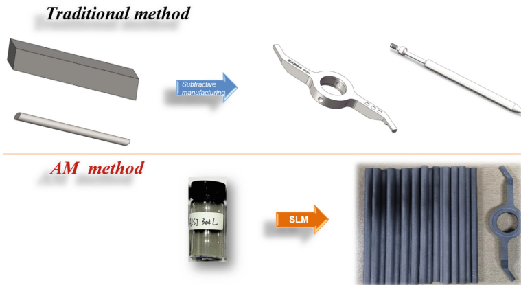
Fig.4. The process diagram of AM compression rod and thimble plug
