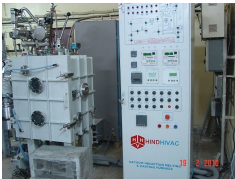
Fig. 10.10 Inductively heated vacuum melting system
