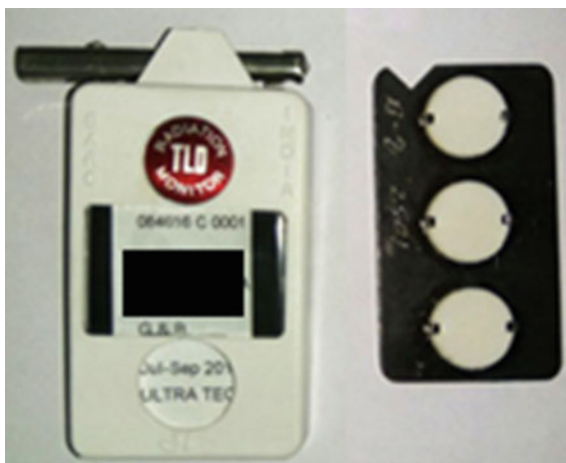
Fig. 10.7 TLD Badge and TLD Card used for country-wide personnel monitoring in India
