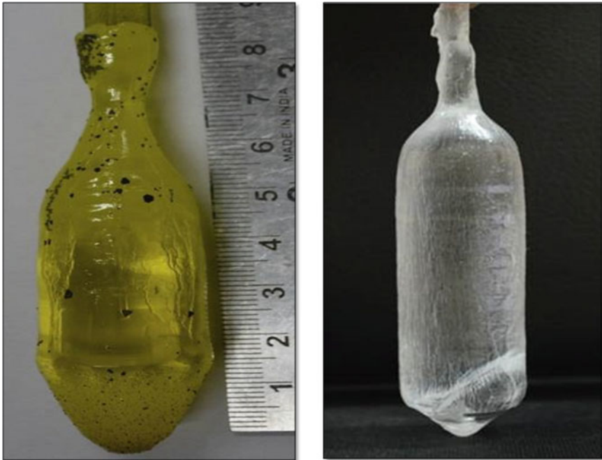
Fig. 22.15 Photograph of a 30 mm diameter and 50 mm length YAG:Ce (Left) and YAP:Ce (Right) scintillator single crystal grown by Czochralski technique at CTS, TPD
