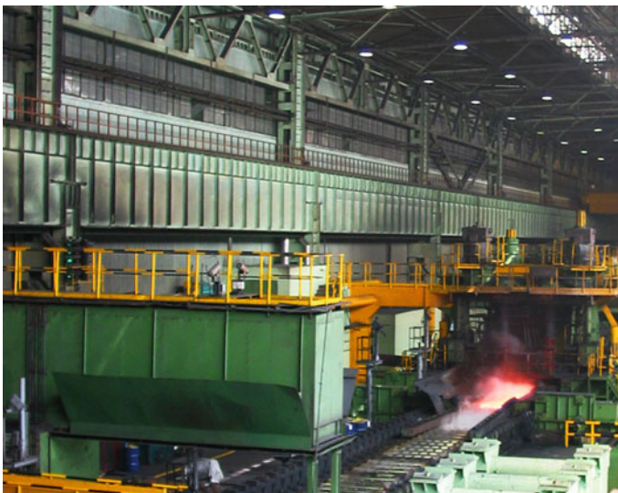
Fig. 7.2 Hot rolling steel. Attribution: Erik Charlton from Menlo Park, USA, CC BY 2.0 https://creativecommons.org/licenses/by/2.0 , via Wikimedia Commons
