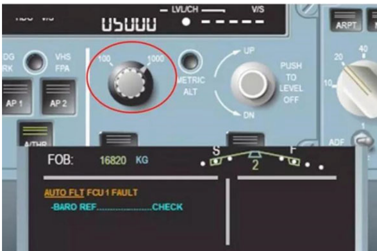
Fig. 28.2 Fault display of FCU on ECAM (Electronic Centralized Aircraft Monitor)
