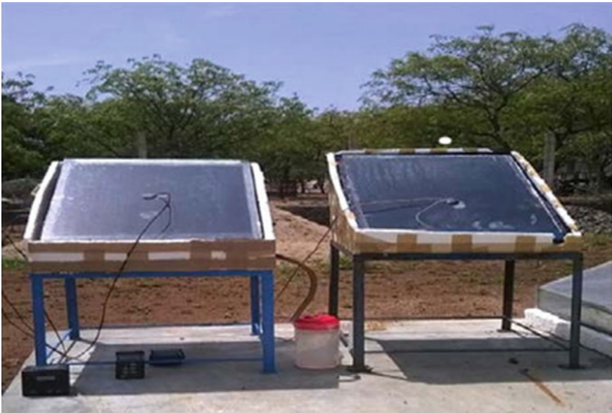
Fig. 7 Image of the experimental setup of solar still [27]
