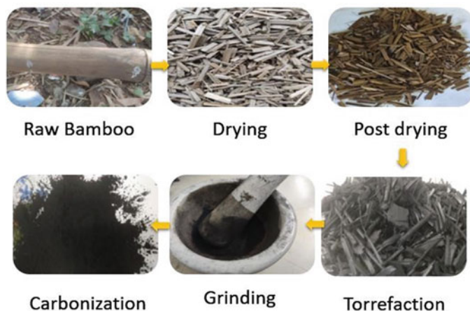
Fig. 1 Schematic showing preparation of BB-400
