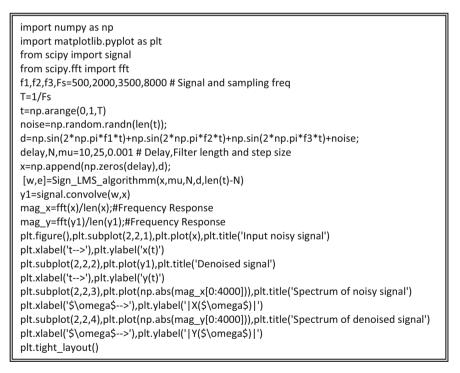
Fig. 11.22 Python code for adaptive line enhancer using sign LMS
