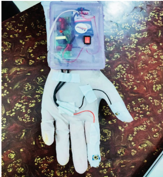
Fig. 9 Prototype testing of shock circuit gloves
