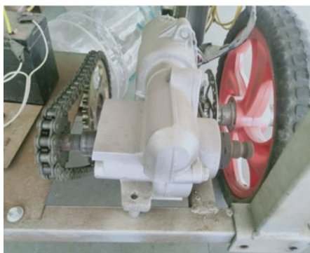
(a) Braking system with the rear wheel
