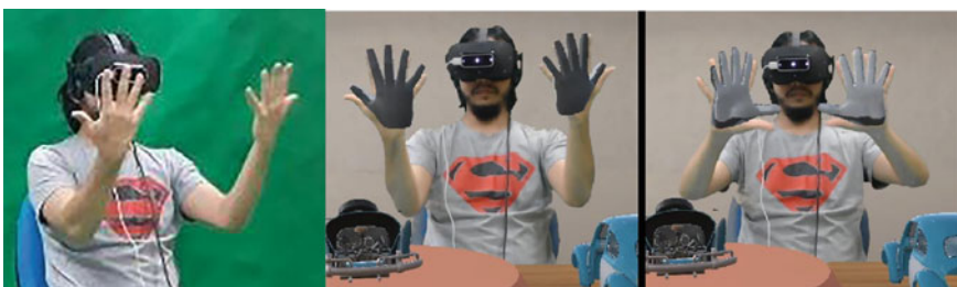
Fig. 2 Palm up and palm down gesture inputs
