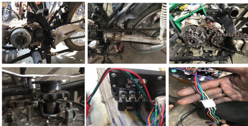
Fig. 6 Assembling of different part of the proposed electric bike
