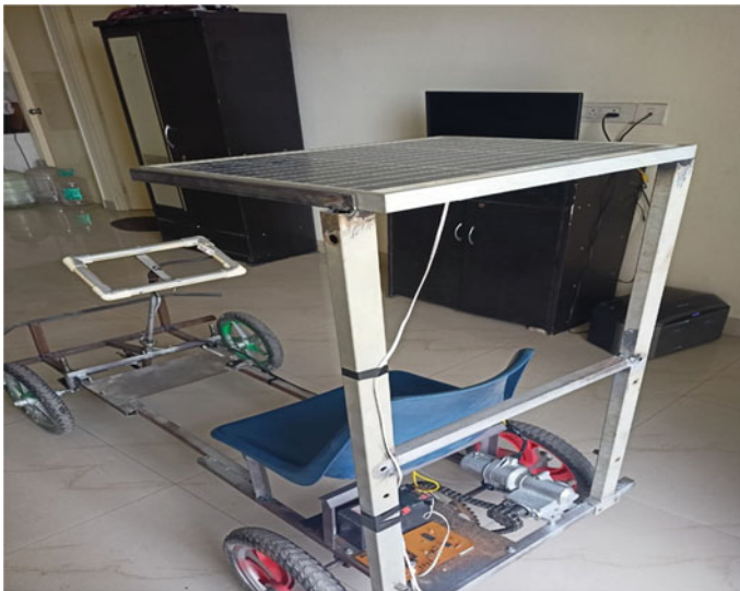
Fig. 4 Overall view of solar charging electric vehicle
