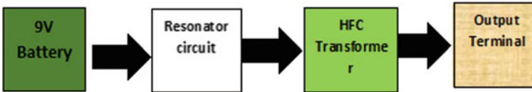
Fig. 3 Electric shock in stun gloves
