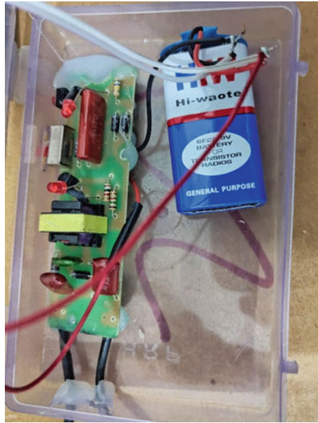
Fig. 8 Electric shock gun implementation
