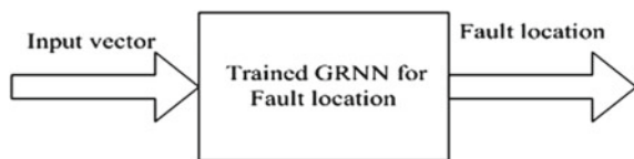
Fig. 2 Block diagram of GRNN-based fault classifier
