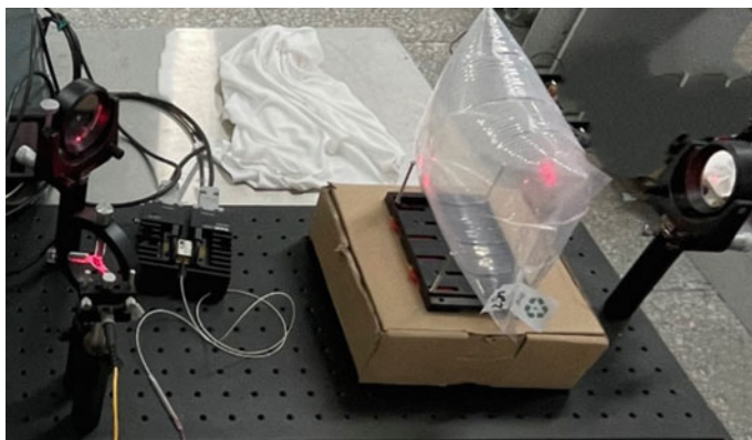
Fig. 16.8 Gas bag simulating a leaked gas plume
