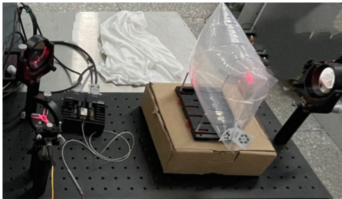
Fig. 16.8 Gas bag simulating a leaked gas plume
