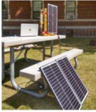
(a) Solar-powered 3D printer [33]
