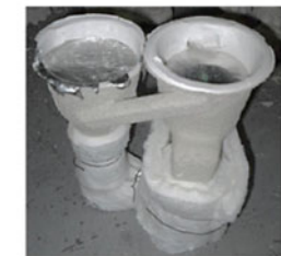
Fig. 12 Investment casting of 3D-printed cellular patterns [21]
