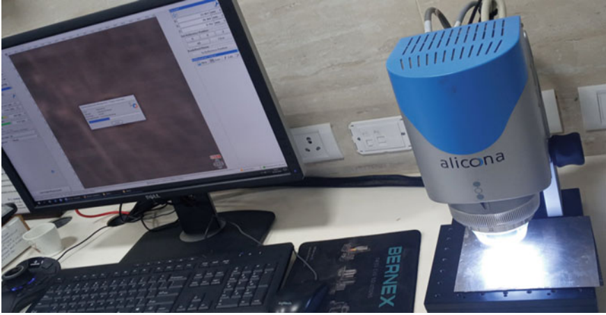
Fig. 2 Measuring diameter of machined micro-holes on work material by ALICONA optical microscope
