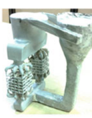
Fig. 12 Investment casting of 3D-printed cellular patterns [21]
