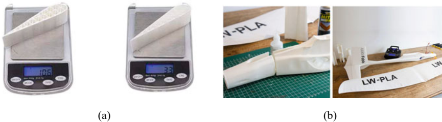
Fig. 2 a Comparison of the weight of parts printed with standard PLA and LW-PLA b printed model of aircraft with LW-PLA. Source ColorFabb [10]
