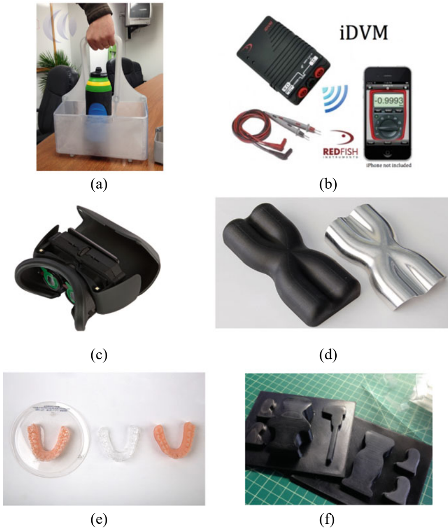
Fig. 10 AM application in rapid tooling for a water carrier: FIFA 2014 [13], b digital multimeter [14], c housings and the exterior cover [15], d hydroformed Diamond [13], e thermoformed aligners [16], f vacuum mould [17], g injection moulds [18], h paper pulp mould [19], i jigs and fixtures [20] and j investment casting [13]
