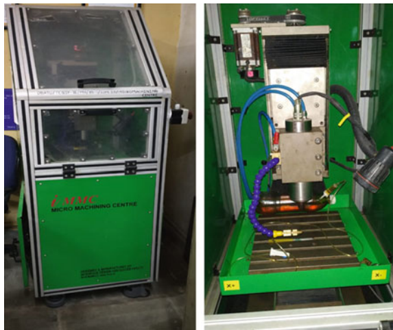
Fig. 1 CNC micromachining station for micro-drilling
