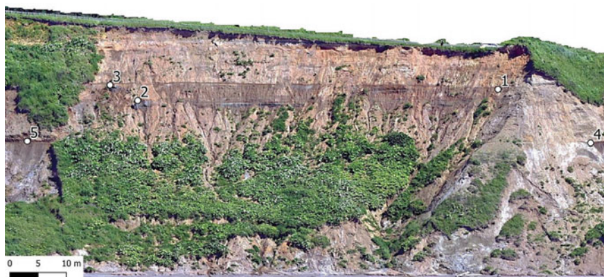
Fig. 2 Orthophotoscheme of the coastal ledge in the Novoselovo village area: 1–3 geological sections with sampling for radiocarbon and facies analyses, 4–5 points for determining the geospatial parameters of the paleobench
