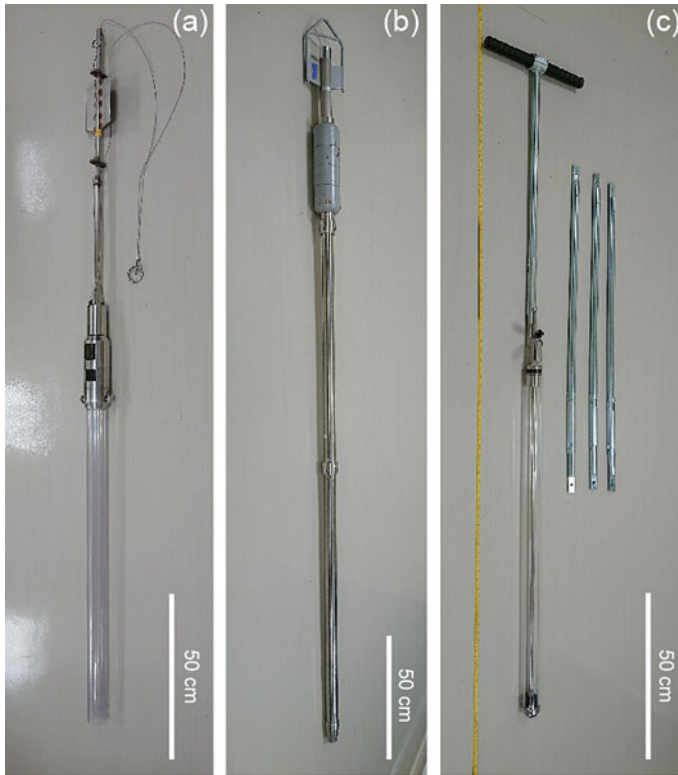
Fig. 10.3 Examples of gravity core samplers ( a and b ) and c a hand-drilled sampler used to obtain relatively short sediment cores
