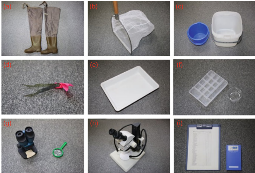
Fig. 11.3 Photographs of survey equipment: a waders, b D-framed net, c buckets, d spring steel tweezers, e white plastic pan, f divided plastic case or plastic cups, g field binocular microscope or magnifying glass, h standard binocular microscope (for laboratory use), and i clip board and tally sheet or water-resistant field book
