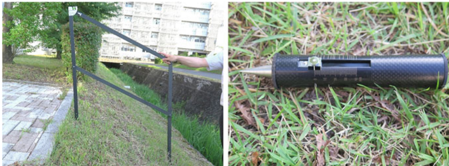
Fig. 12.5 Field survey tools for environmental data collection: gradometer (left) and the Yamanaka soil hardness meter (right)
