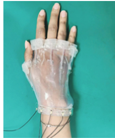
Fig. 5. The ultrasonic waveguide-integrated artificial skin worn on a human hand.
