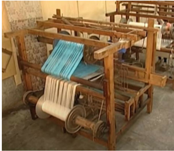
Fig. 4 Double warp beam in a single handloom. Source Historische Handweberei-web MUSEUM OEDERAN
