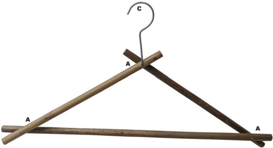
Fig. 10 Ghost: In this variation, the hanger is made collapsible. The hanger consists of three bamboo members and a hook. The corner junctions are riveted. The central junction is held together by the hook itself. It can accommodate all types of garments
