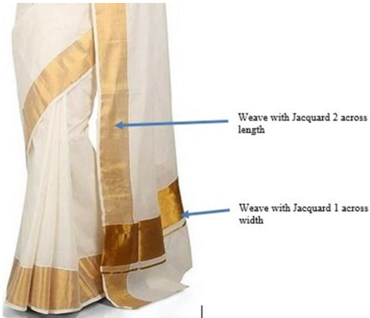
Fig. 6 Fabric ornamentation produced with double jacquard in a single handloom
