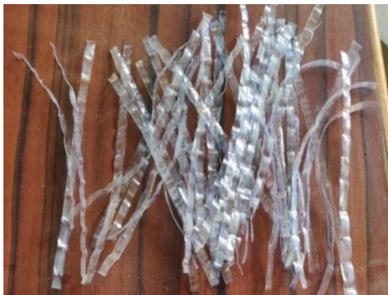
Fig. 1 Plastic strip cut from used plastic water bottles added in concrete cubes
