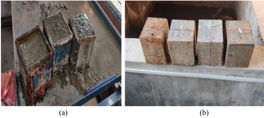
Fig. 2 a Casting of concrete cubes; b curing of concrete cubes
