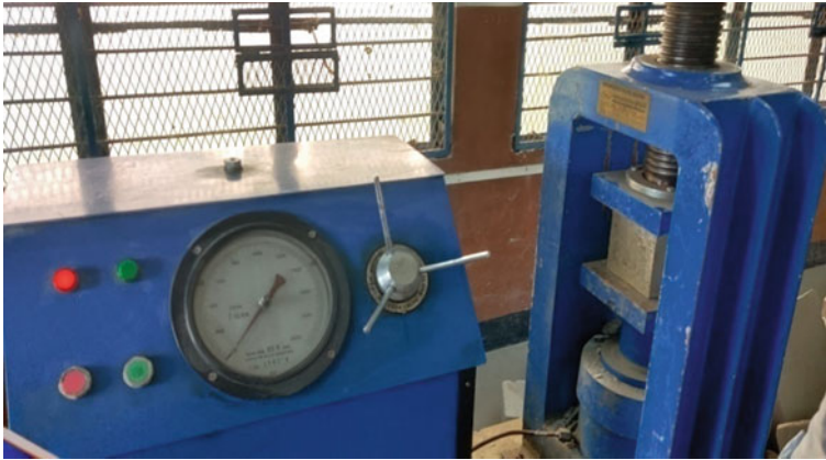
Fig. 4 Experimental set up for compression testing of concrete blocks
