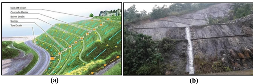
Fig. 5 Slope stabilization with the use of drainage. Source https://youtu.be/At0G2HEgVDo
