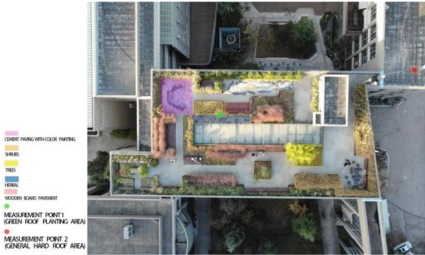
Fig. 2 The measured green roof with different types of ground
