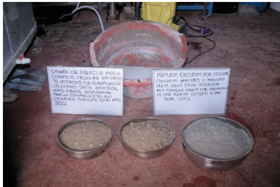
Fig. 1 Materials cement, fine and coarse sand, water and foaming agent (Hydro-Washer)
