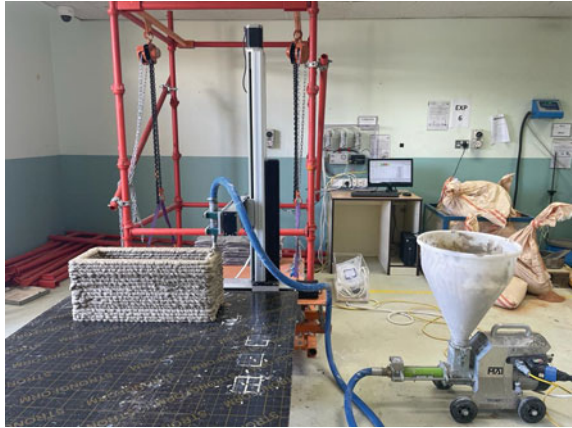
Fig. 4 Concrete 3D printer developed at Sohar University, Oman
