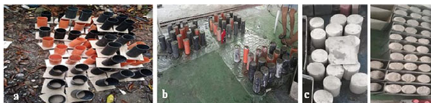
Fig. 1 a Cylinder molds; b Wet concrete cylinders for curing; c Cured concrete cylinders
