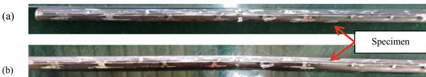
Fig. 9 Non-prismatic pipe specimen. a before buckling experiment; b after buckling experiment
