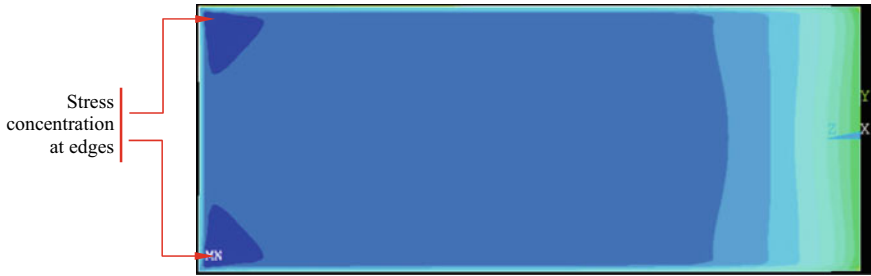
Fig. 5 Stress pattern in the member of problem 1 for the first iteration showing stress concentration at the corners
