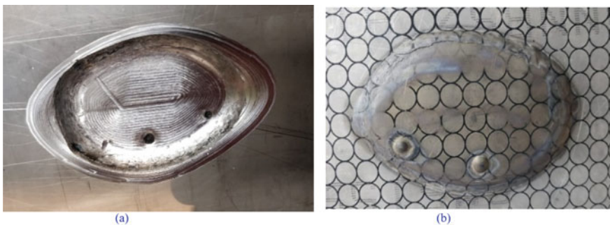
Fig. 4 Failure of sheet due to crack
