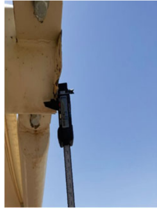
Fig. 4 a Parking structure dimensions (Back parking). b Surveying for parking structure dimensions
