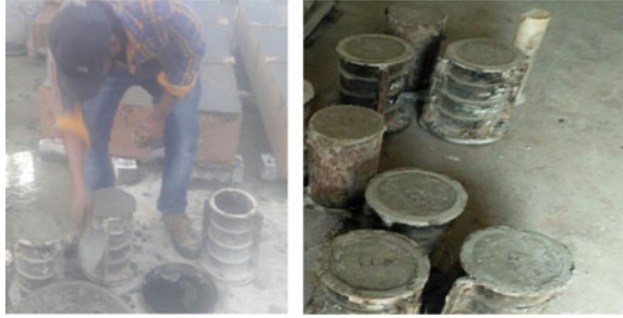
Fig. 4 Cylinders are cast in a mould
