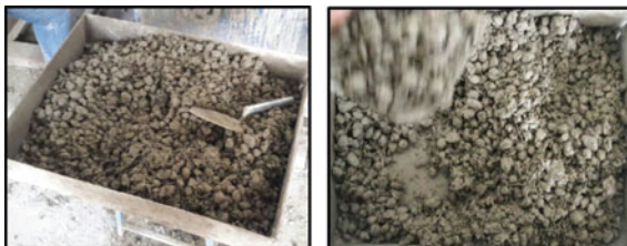
Fig. 2 Marine brown algae concrete
