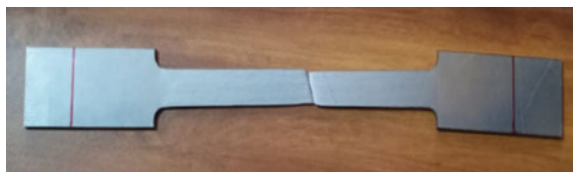
Fig. 5 Tensile testing strip
