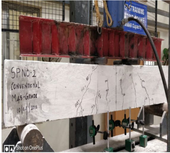
Fig. 14 Deflection testing of beam
