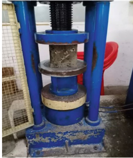
Fig. 4 Compressive strength test
