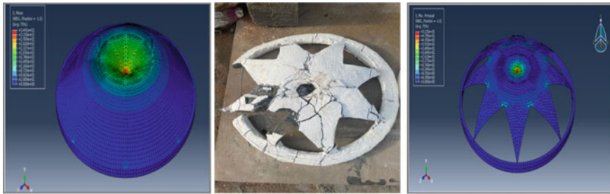
Fig. 17 Failure of conventional and bio-mimicked dome model
