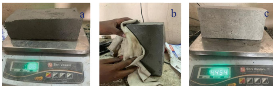
Fig. 2 Water absorption test of sustainable brick a dry weight, b wiping of brick, and c wet weight
