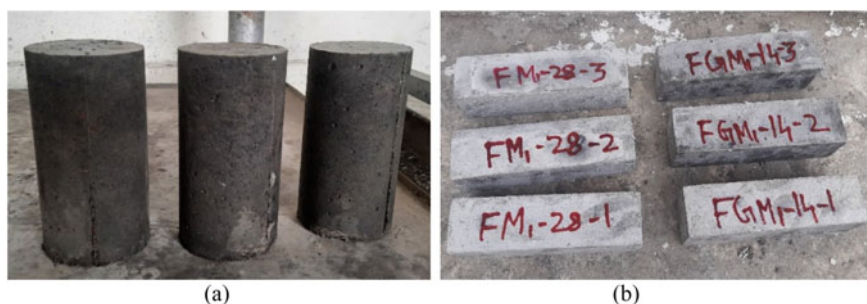
Fig. 1 Specimens. a Static modulus of elasticity. b Dynamic modulus of elasticity
