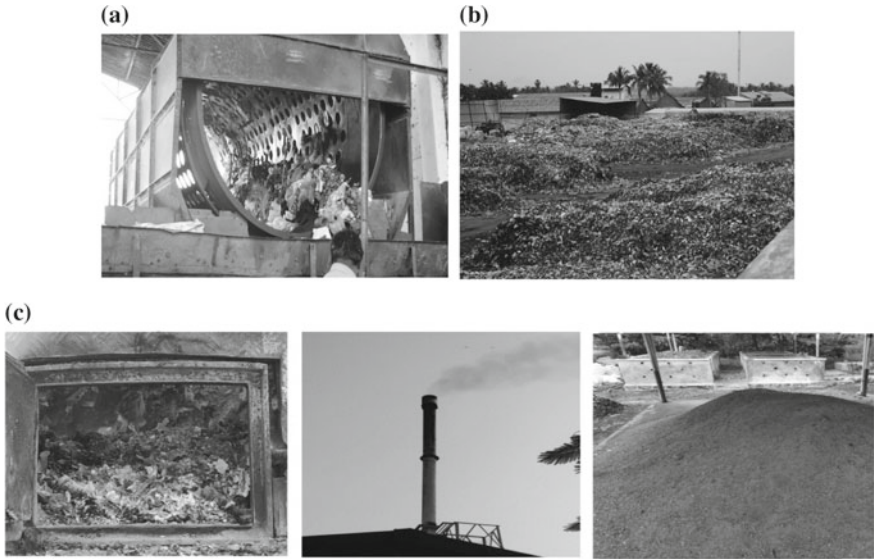
Fig. 1 a Pre-processing in 120 mm sieve. b Heap formation. c Processing of the municipal solid waste in the municipal incinerator plant
