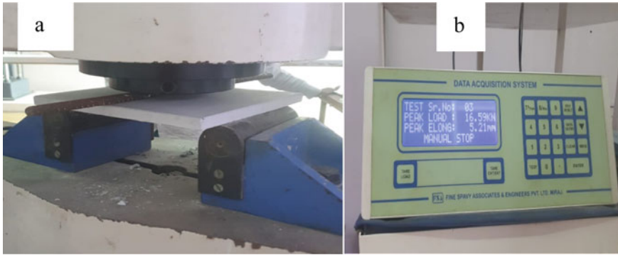
Fig. 3 Shows the experimental test procedure of tiles during modulus of rupture a Apply breaking load, b Digital display of load
