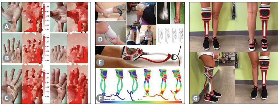
Fig. 3. Application study and evaluation of self-powered flexible e-skin based on ultra-stretchable friction nano-integration. (A) Changes in the current map of the super-stretchable friction nano-integrated self-powered flexible e-skin also clearly show the position of the finger. (B) Response rates of 37% and 49% for monitoring fingers and joints, respectively. (C) Self-powered flexible electronic skin based on super-stretchable friction nano-integration is attached to the palm. (D) Electrostatic induction generates a small number of electrons for electrical signals. (E) The study can be attached to complex surfaces with different bending, folding bending, twisting, and coupling bending. (F) The implementation of the mechanical function of the device sensor was investigated and tested. (G) The self-powered flexible electronic skin with super-stretchable frictional nano-integration ensures the functionality.
