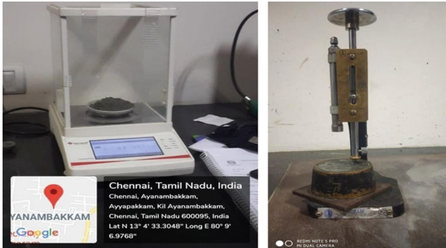
Fig. 1 Specific gravity and setting time test of cement
