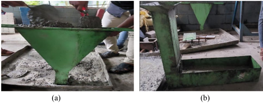
Fig. 1 a V-funnel test; b L-box test
