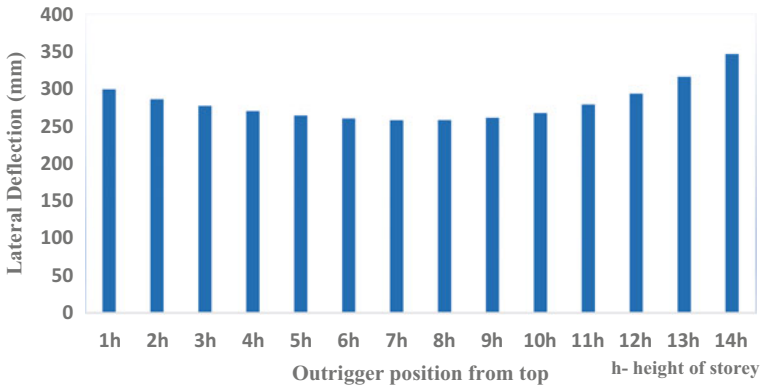
Fig. 4 Maximum lateral displacement of a 15-story frame with single-level outrigger
