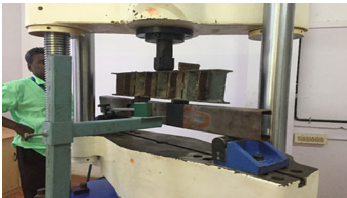
Fig. 5 Flexural testing of retrofitted beam specimen using UTM
