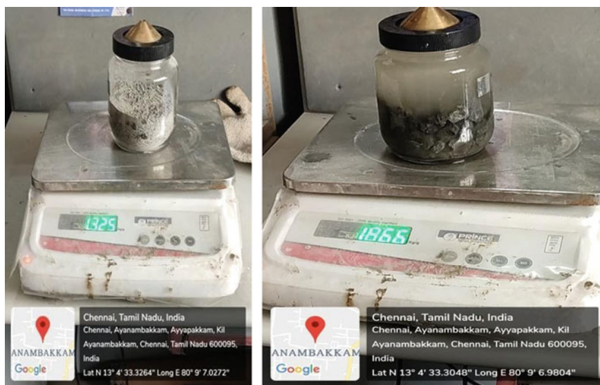
Fig. 2 Specific gravity test of fine and coarse aggregates
