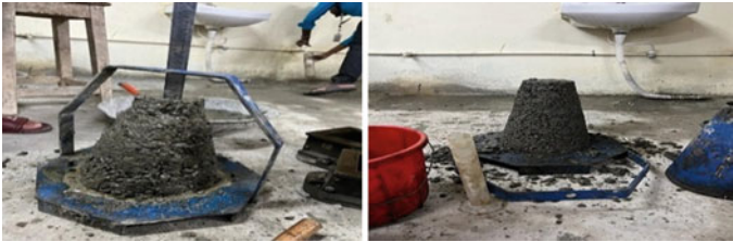
Fig. 2 Slump cone test
