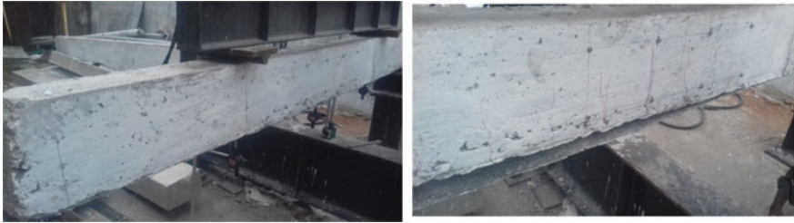
Fig. 3 Failure modes of beam
