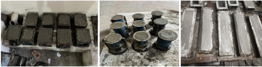
Fig. 1 Casting of cube, cylinder, and prism specimens
