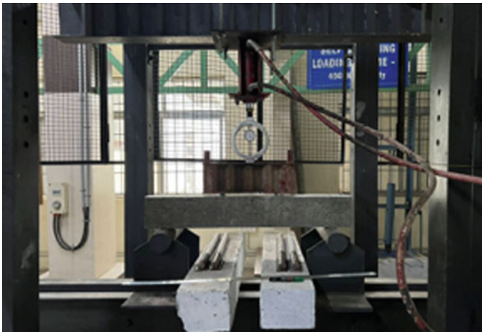
Fig. 7 Testing of the reinforcement beam
