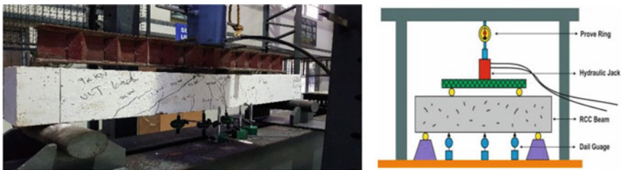
Fig. 19 Load deflection test on RCC beam with steel fibre
