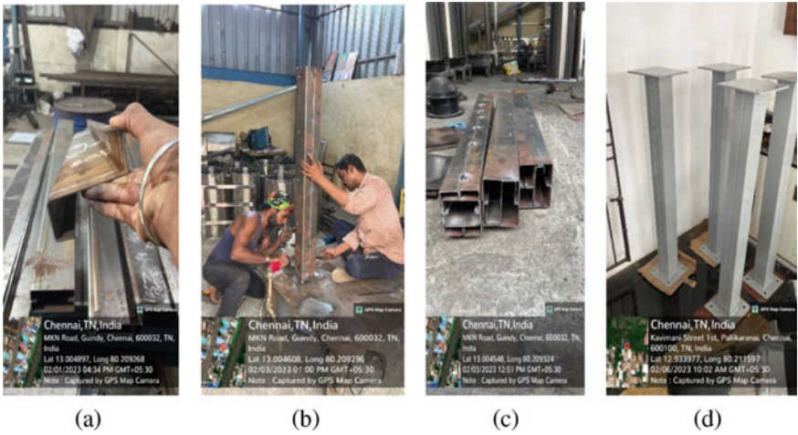
Fig. 6 Fabrication process of columns a Bending; b fabrication; c fabricated models; d protective coating to models
