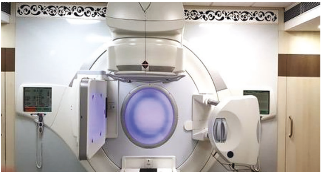
Fig. 1 Linear accelerator with a 160-leaf multi-leaf collimating system allowing for precision shaping of the beam to the target area
