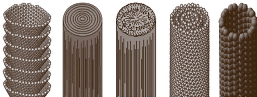
Fig. 4.1 Graphical representation of carbon fibres and carbon nanotubes [26]
